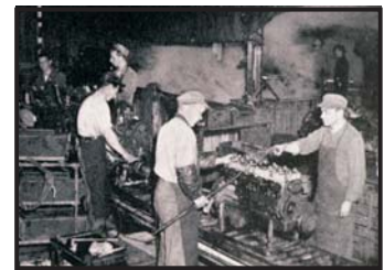
Engines are disassembled, cleaned and component parts separated for further processing in sub-assembly sections.
