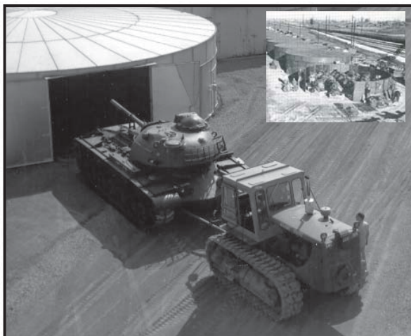
Experimental long-term de-humidified storage tanks were built to "can" or preserve vehicles. With the demands for ordnance materiel, the process is tested and deemed a success as vehicles come out of the 169 petroleum storage tanks -- all in excellent condition.
